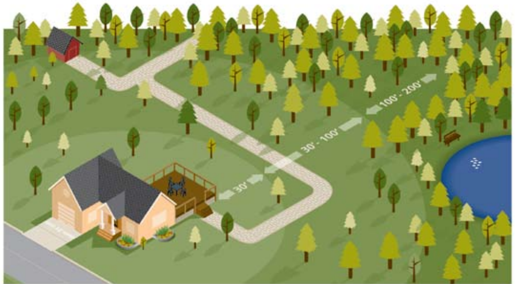
The Home Ignition Zone includes the house and its immediate surroundings within 100 to 200 feet.
